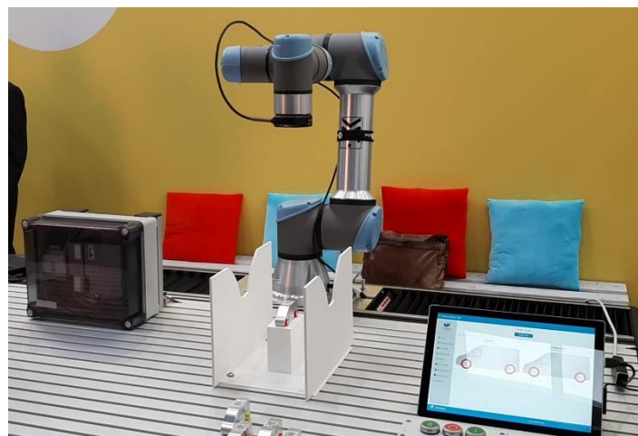
Figure 63: Using the IIP-Ecosphere platform to realize a robot-based visual quality inspection for Hannover Fair 2022.
